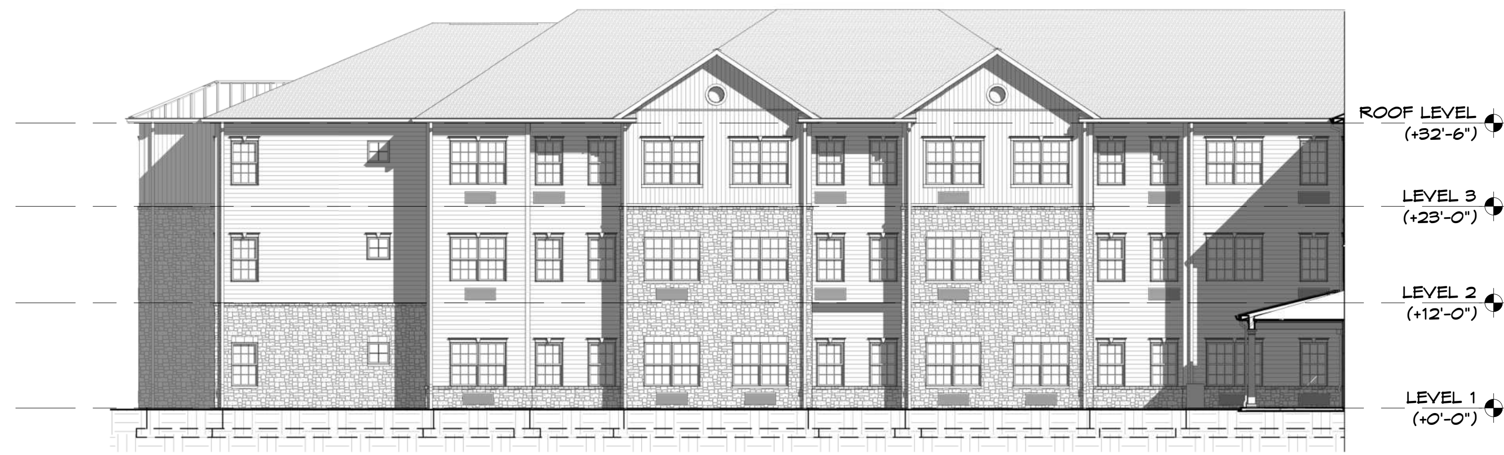
1 T-105 FRONT LEFT INSIDE ELEVATION Scale: 3/32" = 1'-0"
