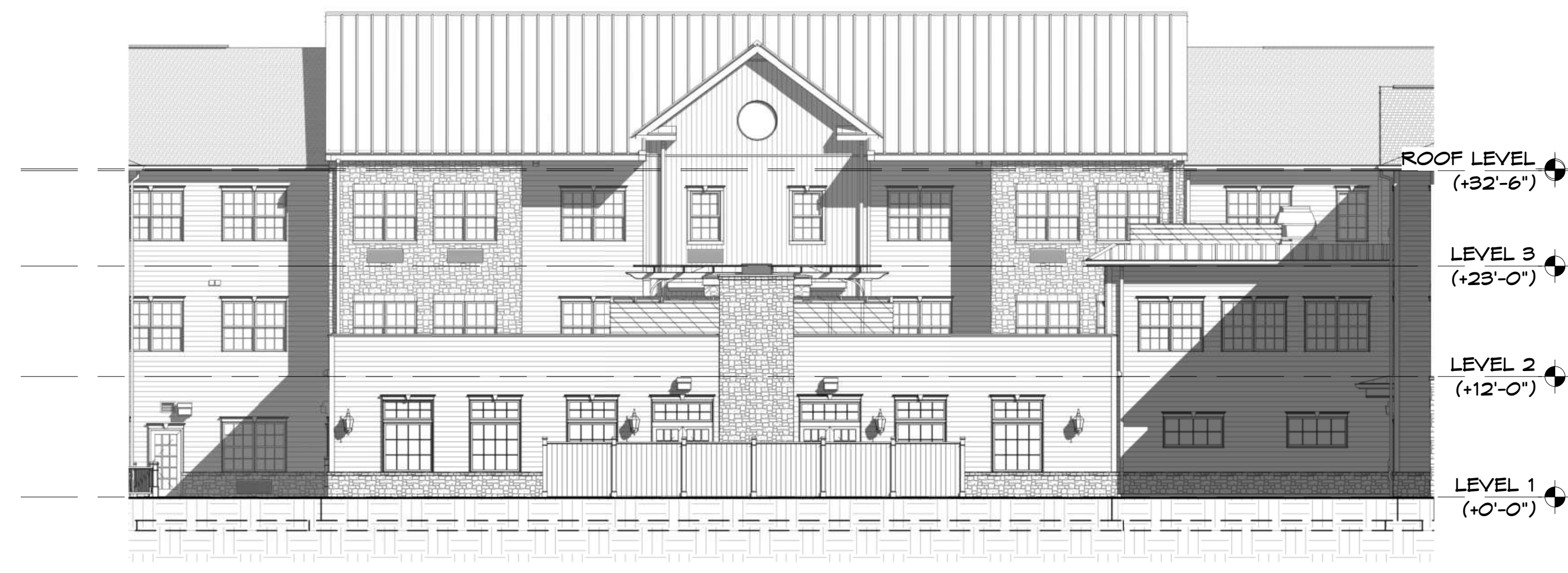
5 T-105 REAR ELEVATION Scale: 3/32" = 1'-0"
